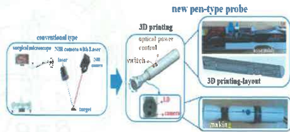
Fig. 4 Fabrication of a pen-type probe using three-dimensional printing technique
