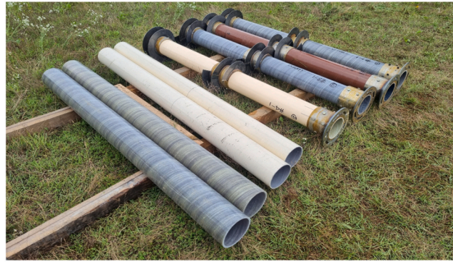
Fig. 3. Fiber-reinforced polymer Screw Pile Specimens.
