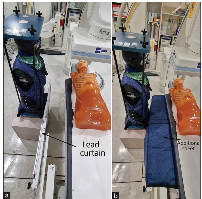
Figure 1: Images of radiation dose measurement with (a) and without (b) the additional shielding sheet placed between the interventional table and lead curtain
