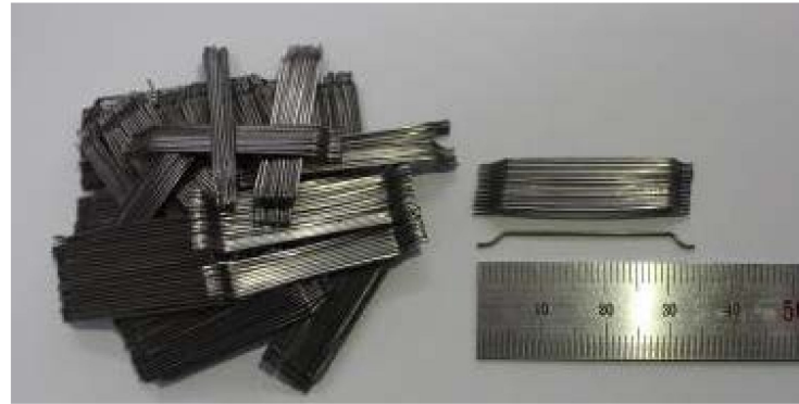
Figure 2. Shape and dimension of steel fiber.
