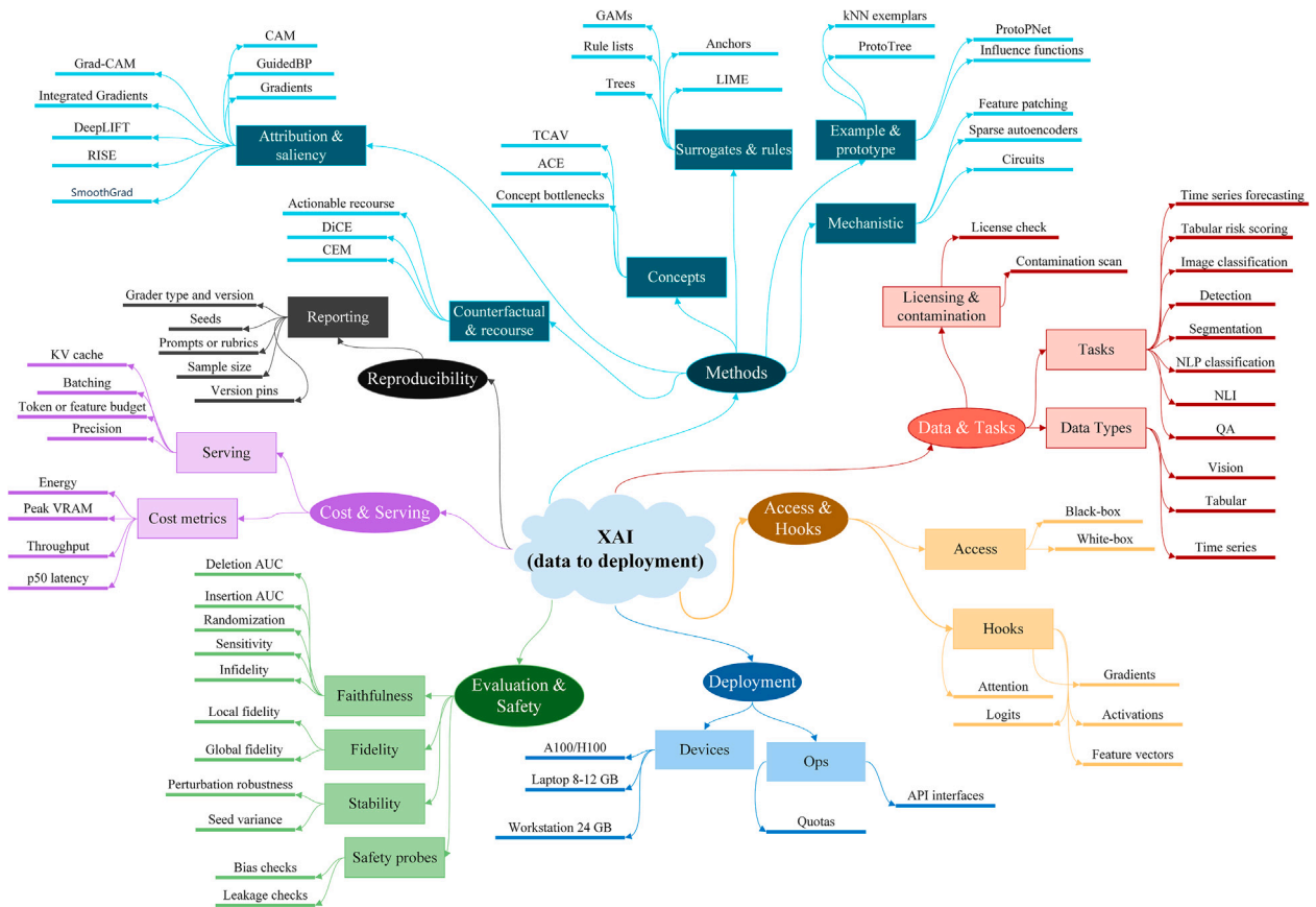
Fig. 2. End-to-end XAI MIND map organizing the full pipeline from data types and tasks through model access and hooks, explanation method families (attribution and saliency, surrogates and rules, counterfactuals and recourse, concepts, examples and prototypes, mechanistic analyses), evaluation and safety metrics (faithfulness, fidelity, stability, safety probes), reproducibility reporting, serving parameters, and deployment environments. The map serves as a navigation guide connecting method selection to the evaluation protocol and deployment context.
