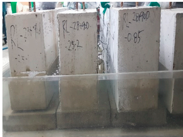
Figure 7. Partial water curing of pre-damaged test members.
