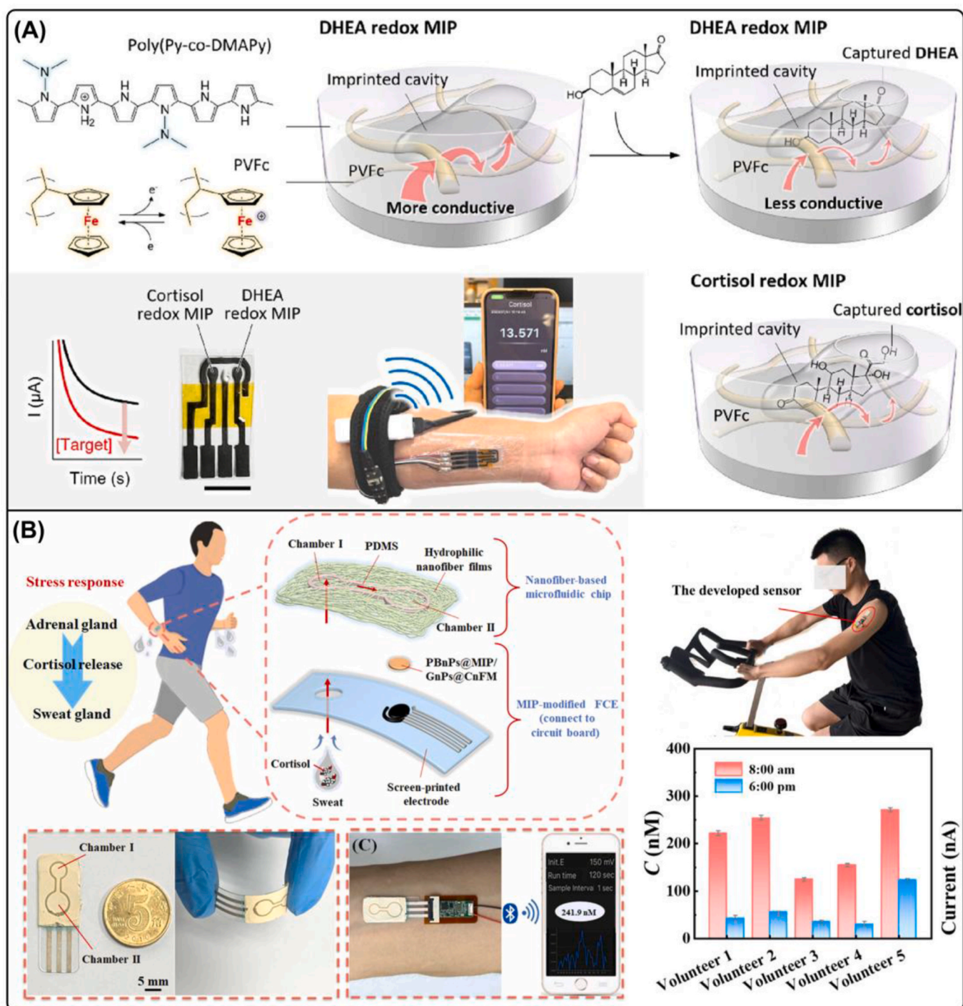
Fig. 4. (A) Redox-active MIP sensing strategy and wearable implementation. Reproduced with permission from Ref. [105]. (B) Schematic design, wearable integration, and on-body evaluation of a flexible cortisol sensor. Reproduced with permission from Ref. [106].
